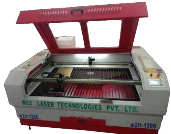
CNC Laser Engraving and Cutting Machine
